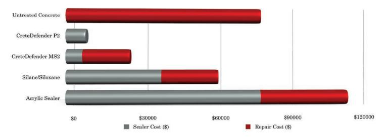
Comparison of 25-year life costs of 10,000 square feet of concrete, including re-application and repair costs determined by product failure rates. Data from Life-365™ concrete analysis software.
